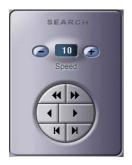
**Search Tools:** Buttons in upper line works for fast rewind (left directional arrow) and fast forward (right directional arrow). Buttons in middle line activate the normal playing back in forward and reverse but the speed can be adjusted by controlling ( - ),( + ) tabs on the top. The buttons in lower line give playback frame by frame, forward or reverse.
