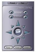
: PTZ cameras connected to DiViS DVR system can be controlled from DiViS Net.
