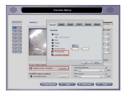
Exit "System Setup" and enter "Color & Motion" configuration under "Camera Setup." Check "Detective motion – Notification". Click on "Properties", and check "Remote Notify" to send notifications when an event occurs. Check "Use Notify Schedule" to utilize the schedule to notify the DiViS Net. If selected, notification schedule on the following page must be configured.
