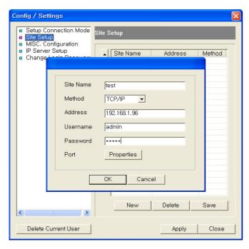
• Site name: Assign system's name or site name. In the use of IP Server, input the Code number as set at "Use IP Server" in the DiViS DVR Setting (DiViS DVR Setting > System > Allow Remote Connections > Properties).
