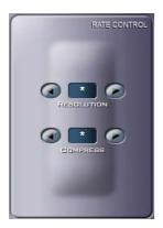
: Compression Rate can be adjusted between 10  $\sim$  90 to enhance the transmission speed (\* for default compression rate). Lower compression rate will provide faster transmission. Resolution can be selected among  $\frac{1}{2}$ ,  $\frac{1}{4}$ , or  $\frac{1}{8}$  (\* for default resolution), and lower resolution provides faster transmission speed. Compression rate and resolution adjusted here are not changing actual resolution and compression rate recorded on the server.
