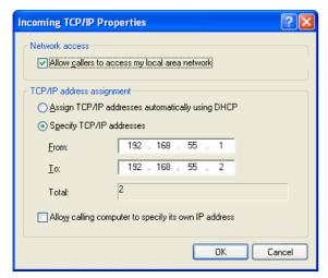
Check "Allow callers to access my local area network". In TCP/IP address assignment, check "Specify TCP/IP addresses", and fill out from and to IP address as shown in picture. It is strongly recommended to use the given TCP/IP addresses. Click "OK", and click "Next" at the Networking Components.
