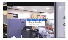
**Save as Movie Clip:** check to create MP4 format movie clips and manually unchecked to stop. The recording is saved at the location assigned from AVI Path. (Refer to 4-1-3. MISC. Configuration for detail) *Note: Recording will cease automatically when the DiViS Net software is minimized.*
