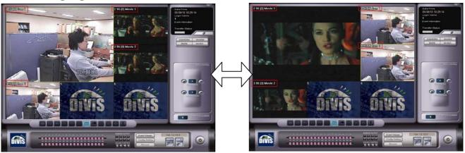
At the connection of DiViS Net software, connected cameras will be positioned in order of camera numbers. It is possible to relocate the camera position to the desired location by left clicking on the image that needs to be relocated, dragging it to the new position, and releasing the left mouse button.
